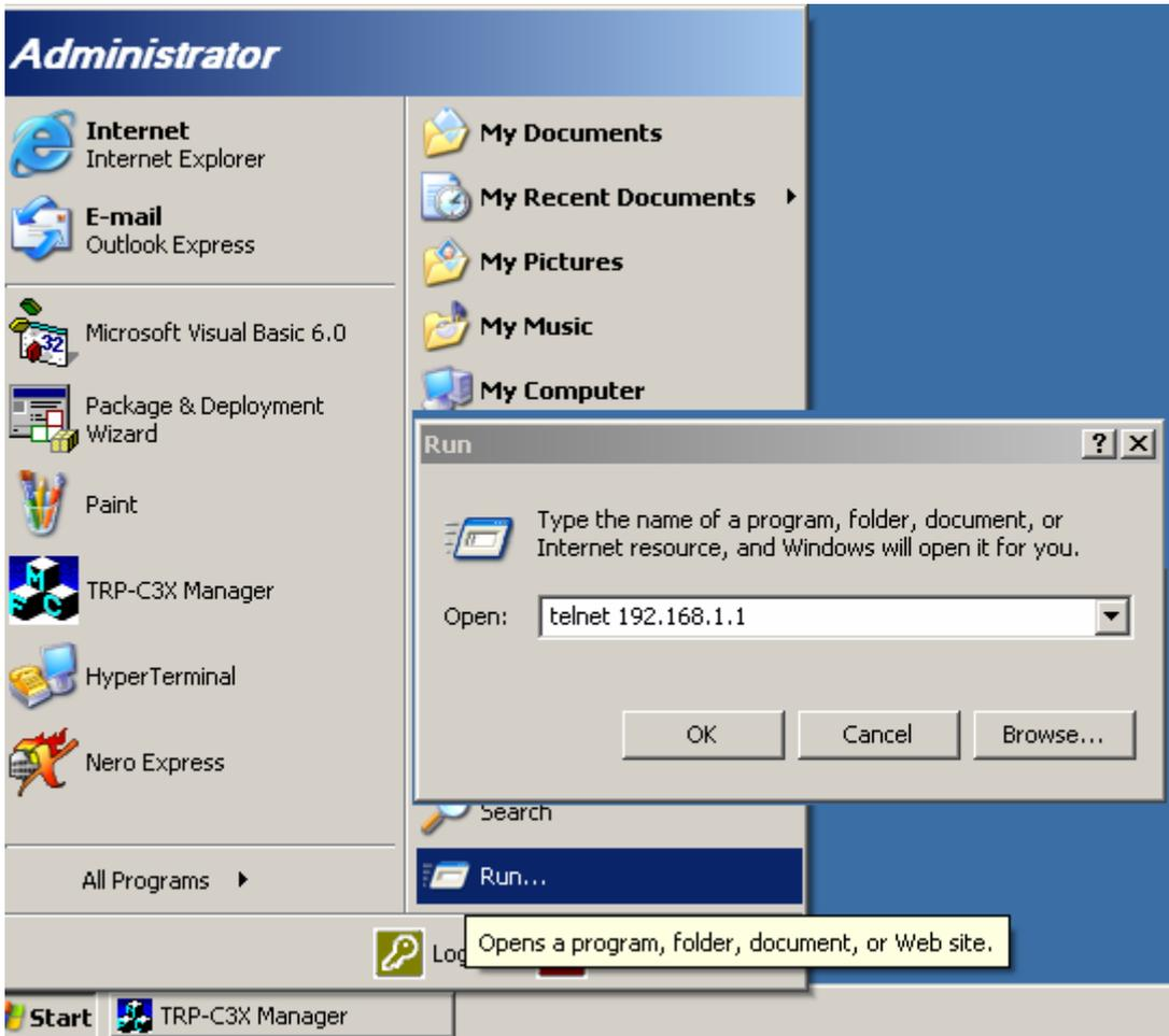
**STEP2.** Click the “OK” TRP-C31M firmware setting will show as following screen. You can set the TRP-C31M by Telnet mode.
