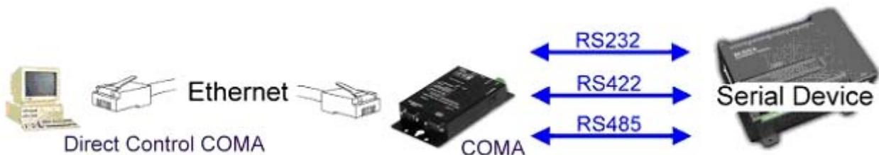
Once the connection is made, the LAN is transparent to the serial device. Applications work just as if the serial device is connected a host's physical COM port. The virtual COM port converts the application's data into IP packet destined for the TRP-C32, which in turn converts the IP packet back to serial data.
