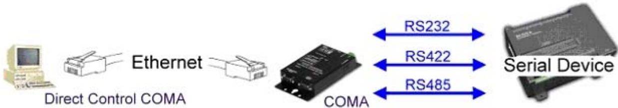
Once the connection is made, the LAN is transparent to the serial device. Applications work just as if the serial device is connected a host's physical COM port. The virtual COM port converts the application's data into IP packet destined for the TRP-C34, which in turn converts the IP packet back to serial data.
