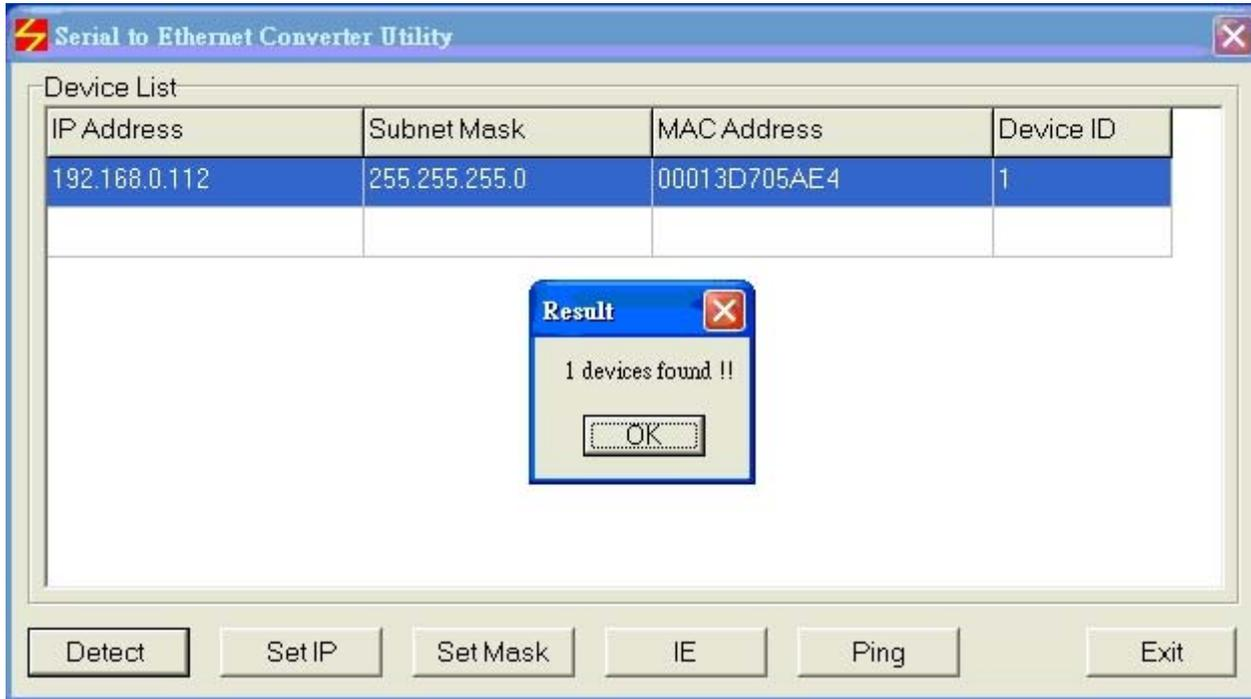
If TRP-C36 was improperly installed it will not be found or detected.
