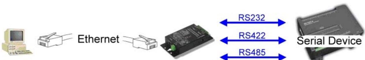
The Virtual COM mode requires the installation of a virtual COM port device driver. In this mode, the TRP-C36 must be set to either TCP/server or UDP/server in the menu with a designated communication port number.
