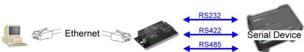
The Virtual COM mode requires the installation of a virtual COM port device driver. In this mode, the TRP-C36 must be set to either TCP/server or UDP/server in the menu with a designated communication port number.
